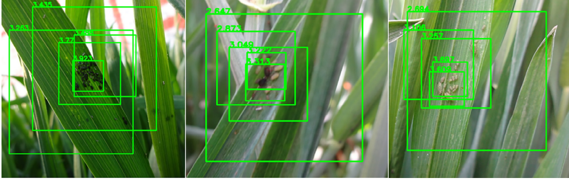
Fig. 7. ClusRPN under-performs due to insufficient training(enlarged for visualization). We find that the network has already been able to select dense cluster areas correctly, but there is a significant deviation of density level prediction. The predicted density levels of low-density areas are much higher than their ground-truth, which causes the size of the final proposed regions to become larger.
