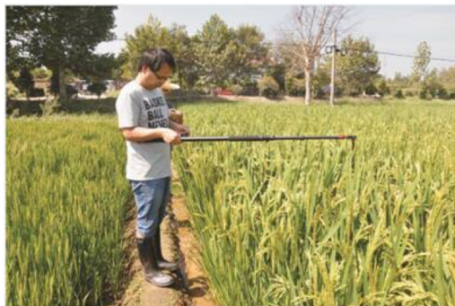
Fig. 9. Wild pest image acquisition equipment and its usage. (1) CCD camera; (2) carbon fiber telescopic rod; (3) mobile client. The parameters of CCD camera are set to 4 mm focal length with an aperture of f/3.3. CCD camera is used to collect pest images and is controlled by mobile client. The position of field would be located by global positioning system.
