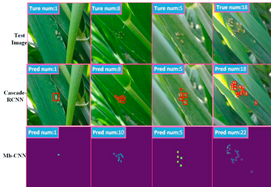
Fig. 11 – The results of low density. There have lower missing and false detection rate by using detection-based method in the case of low density distribution.
