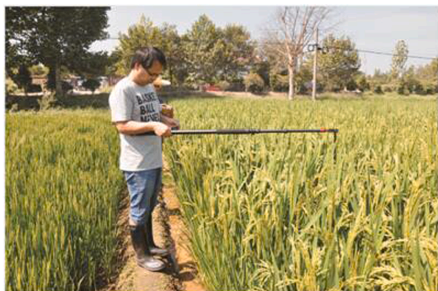
Fig. 4. The usage of rice planthopper intelligent collection equipment in the field.
